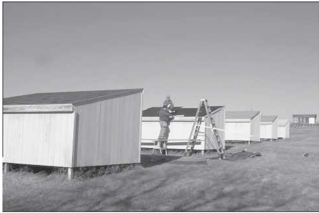
Figure 1. — Exposure structures located at FPL test site near Madison, Wisconsin. All five units were similarly constructed except for roofing materials and were instrumented for long-term temperature monitoring of roof assemblies. Shown from the foreground are black fiberglass shingles, western redcedar shingles (being installed), wood-thermoplastic composite shingles (two structures—closer with lath, further without lath), and white fiberglass shingles.
